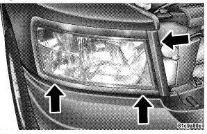
3. Grasp the headlight and pull firmly to disengage the headlight housing from the fender panel.
